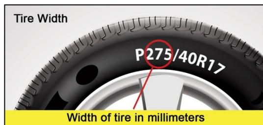
**Tire Width** is the measurement from the widest point of its outer sidewall to the widest point of its inner sidewall when mounted and measured on a specified width wheel. It is measured in millimeters. In this example, the width of the tire is 275 mm.
