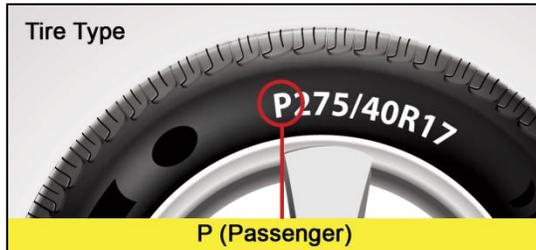
**Tire Type.** The letter “P” at the beginning of the tire size indicates that the tire is a P-Metric tire, referring to tires made to certain standards within the United States, intended for passenger vehicles. The use of P-Metric sizes began in the late 1970s and they are the most frequently used type of tire size today.
