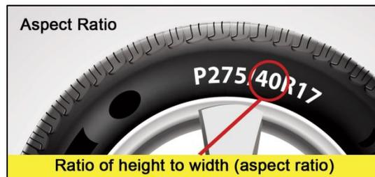
**Aspect Ratio** is the ratio of the height of the tire's cross-section to its width. For example, in a P275/40R17 tire, the 40 means that the height is equal to 40% of the tire's width. The bigger the aspect ratio, the bigger the tire's sidewall will be.
